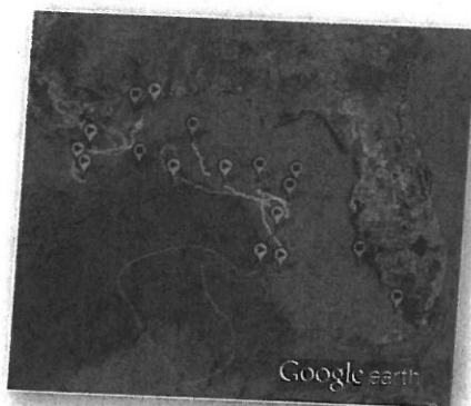
(b) Movement of the drifters with surface currents helped scientists track and predict the movement of oil.
