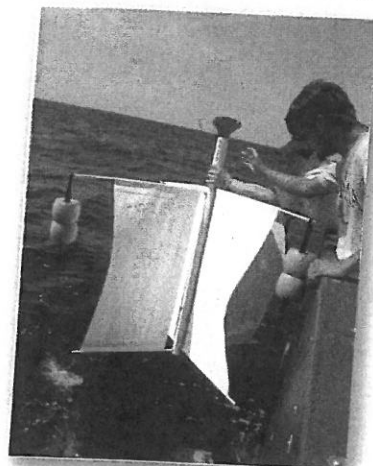
(a) Students deploy a "drifter" (with GPS unit attached to the top of the mast) in the Gulf of Mexico in 2010.
