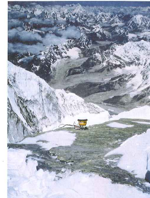
FIGURE 1.19 GPS used to measure Everest’s summit height.
